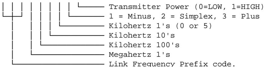
NOTE: To READ or LOAD a link frequency, dipswitch 3 and dipswitch 5 or 6 must be turned ON.
